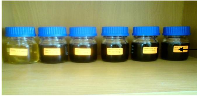
Effect of 40 minutes homogenization process where it can be clearly seen that CNT are uniformly dispersed within the fuel blend for all samples
