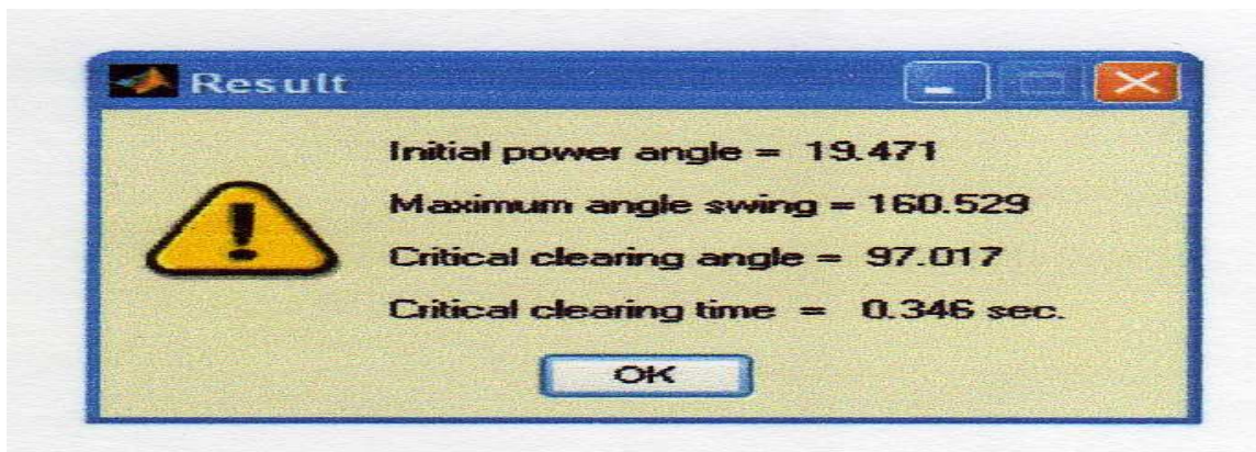
Figure 4.7: The simulation of equal area criterion applied to critically cleared system due to 3 phase fault occurs at the sending end of the line after the user entered the important parameters.
