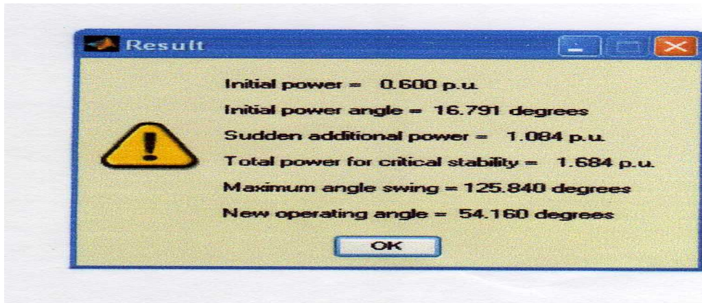
Figure 4.5: The calculated results that related to equal area criterion applied to sudden change in power after the user entered the important parameters.
