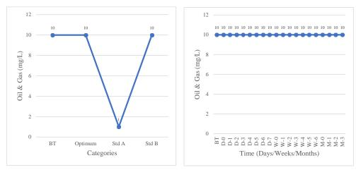
Figure 6. Oil and grease values before and after treatment. BT: Before Treatment, D: Day, W: Week, M: Month
