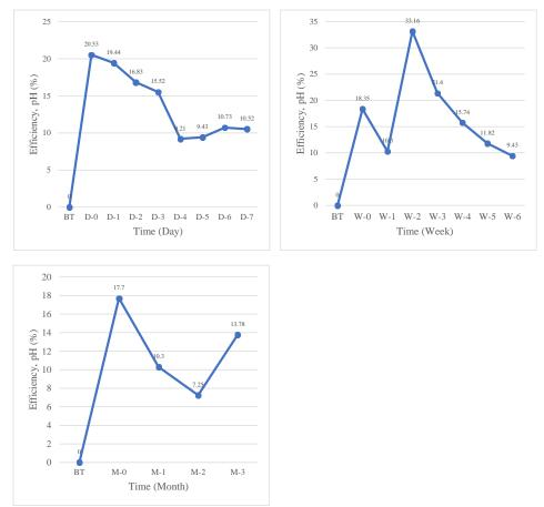
Figure 11. Storage Time Efficiency and Aging Factor of Bio-coagulant in Reducing pH. D: Day, W: Week, M: Month
