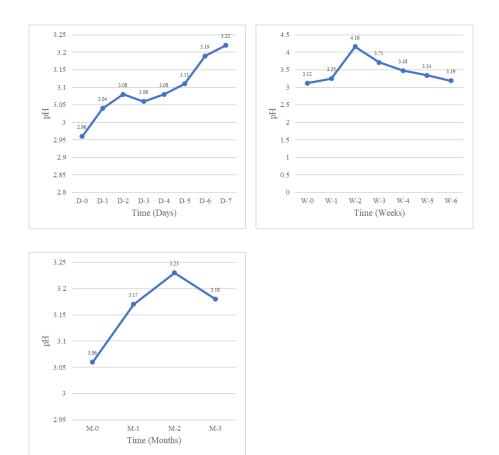
Figure 7. Aging Effect of Bio-coagulant on pH Values. D: Day, W: Week, M: Month
