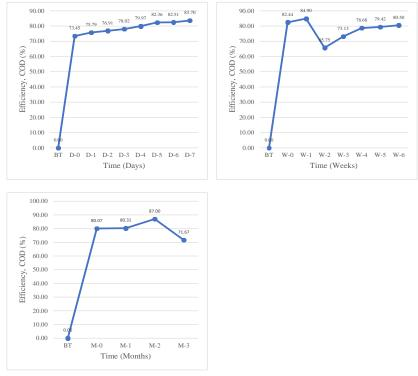
Figure 12. Storage Time Efficiency and Aging Factor of Bio-coagulant in Reducing COD. D: Day, W: Week, M: Month
