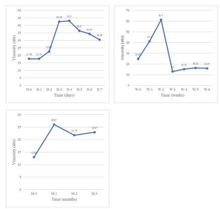
Figure 9. Aging Effect of Bio-coagulant on Viscosity. D: Day, W: Week, M: Month
