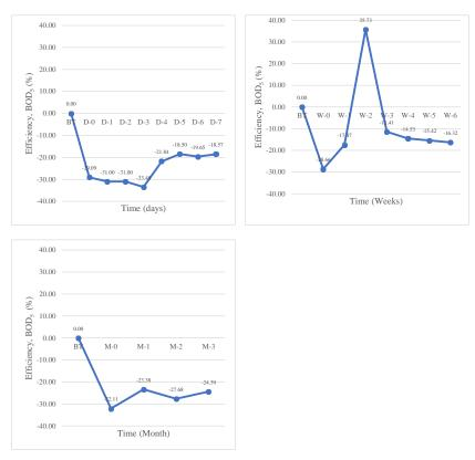
Figure 13: Storage Time Efficiency and Aging Factor of Bio-coagulant in Reducing BOD5. BT: Before Treatment, D: Day, W: Week, M: Month
