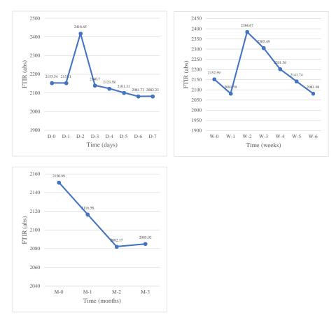
Figure 8. Aging Effect of Bio-coagulant on FTIR Absorbance. D: Day, W: Week, M: Month
