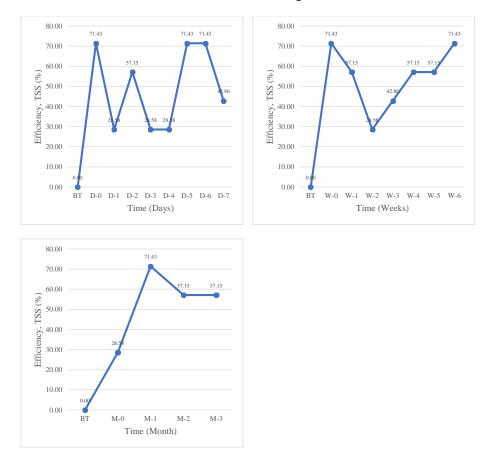
Figure 14. Storage Time Efficiency and Aging Factor of Bio-coagulant in Reducing TSS. BT: Before Treatment, D: Day, W: Week, M: Month
