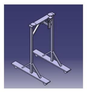
Figure 7: 3D drawing of welding assembly tools
