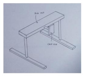
Figure 6: Sketch of assembly tool design
