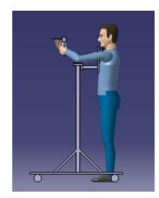
Figure 9: Side view of welding assembly tool
