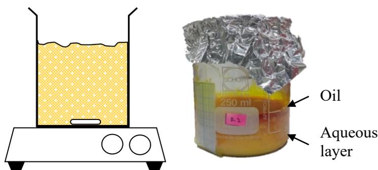
Fig. 1. Heated, stirred beaker for reactive mixing and settling of SS and CPO
