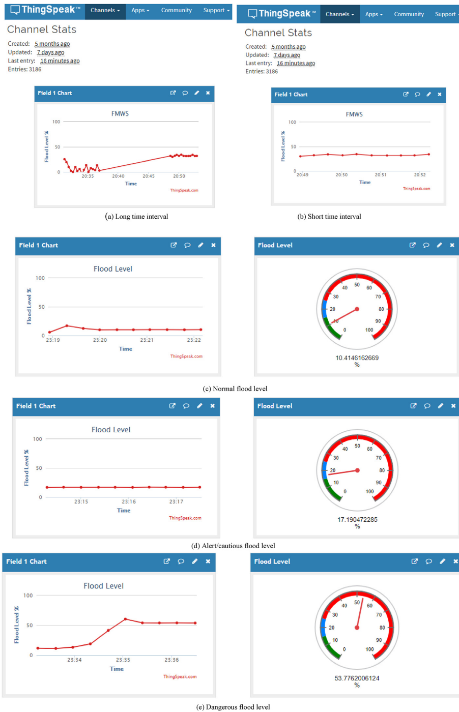
Fig. 9. Flood level measurements extracted from ThingSpeak IoT Channel.
