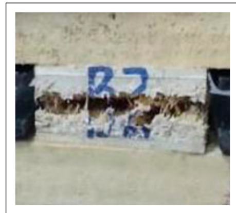
Figure 8. Failure type of blockboard tension load.
