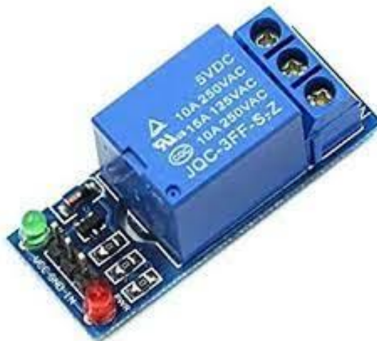
Figure 3.19 One channel relay
