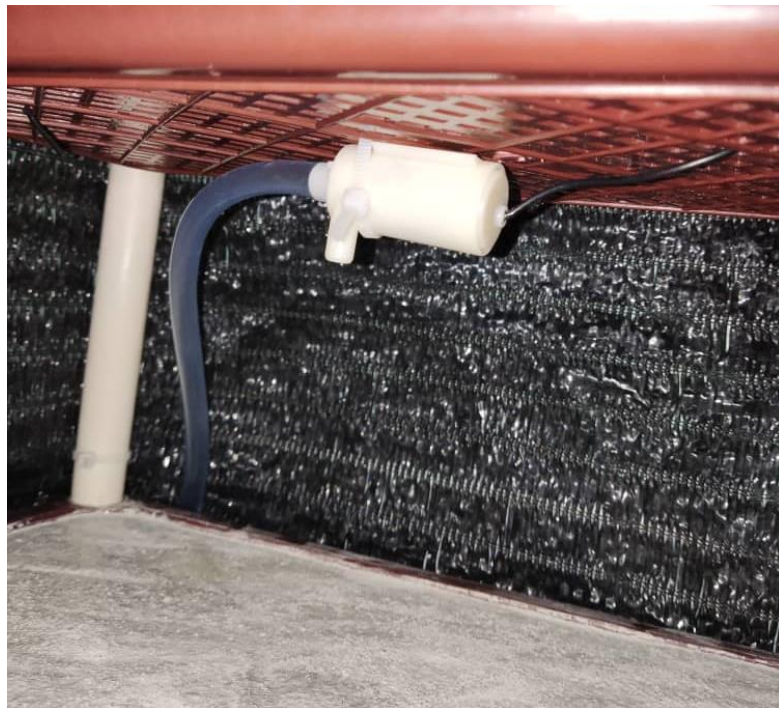
Figure 4.25 prototype diagram (Water Pump placement)
