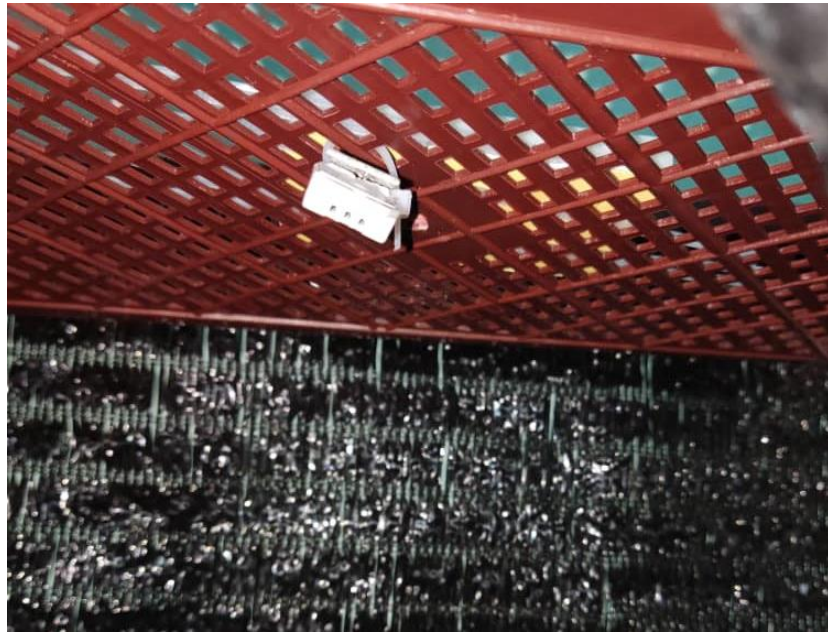
Figure 4.24 prototype diagram (DHT22 Sensor placement)
