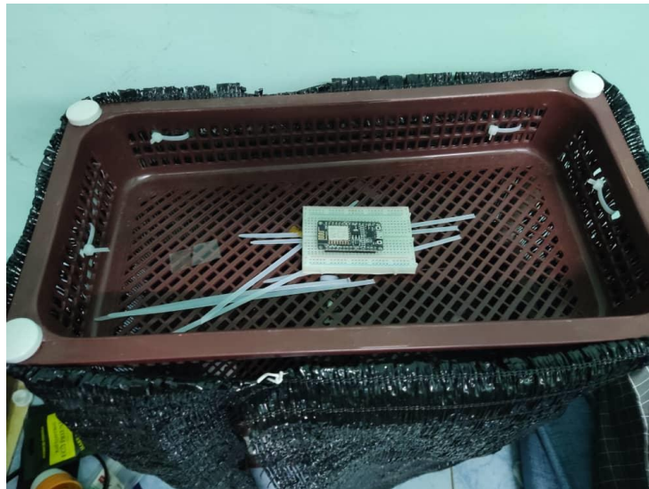
Figure 4.23 prototype diagram (node mcu esp8266 placement)
