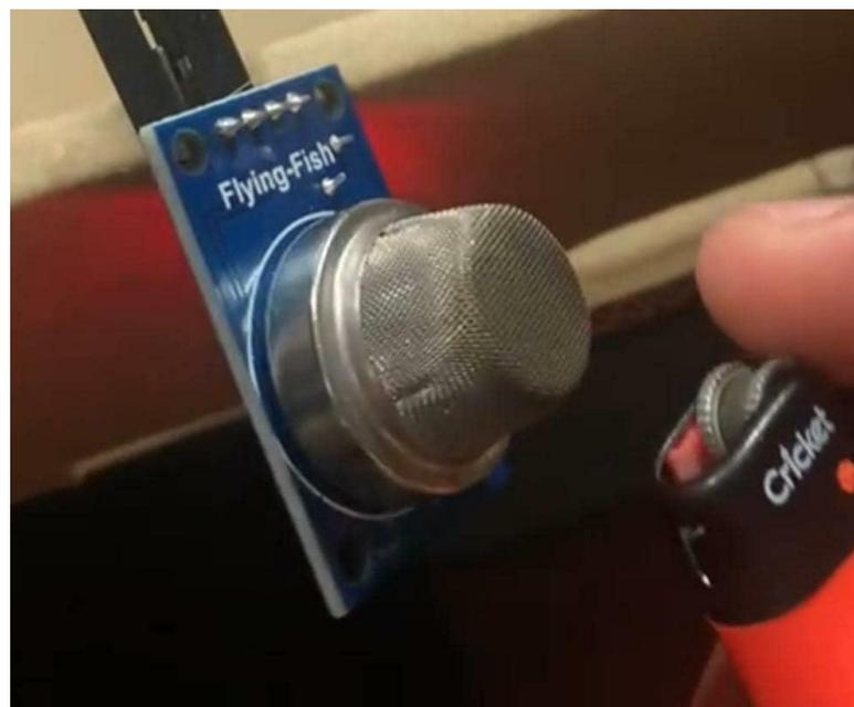
Figure 4.13 : Testing of the gas sensor
