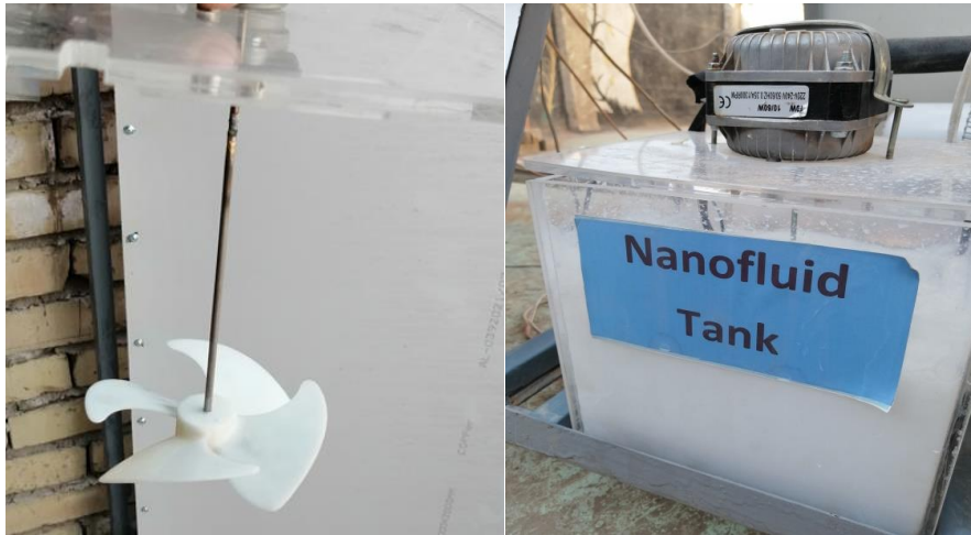
Fig. 5. The stirrer part has been attached to the nanofluid tank.
