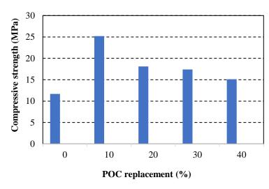
Figure 4. Compressive strength of mortar containing various percentages of POC
