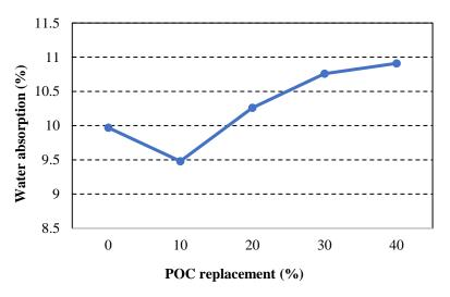
Figure 5. Water absorption in mortar with varying percentages of POC
