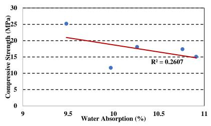
Figure 6. Relationship between compressive strength and water absorption
