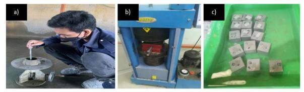
Figure 2. List of experiments a) Flowability test b) Compressive strength test c) Water absorption test
