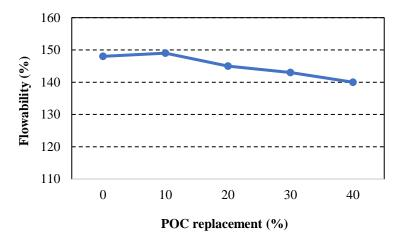
Figure 3. Flowability of mortar containing various percentages of POC
