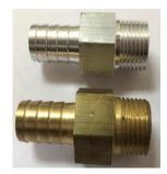
Figure 2. Actual case study product with hole depth 55.00mm.
