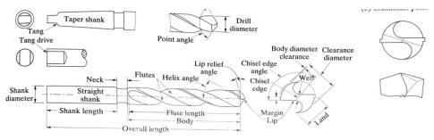
Figure 1. Twist drill part name [4].
