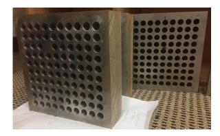
Figure 3. One hole cannot be drilled because the center drill 3.00 mm diameter tool broke down in the Aluminum 6061 workpiece.
