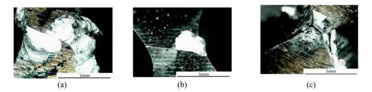
Figure 5. Ghasemi et al. [13] reported the drilling tool worn at the tip.
