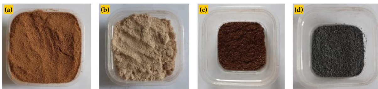
Figure 1. Powder of composites materials: (a) coconut fibre, (b) wood, (c) copper, and (d) aluminum
