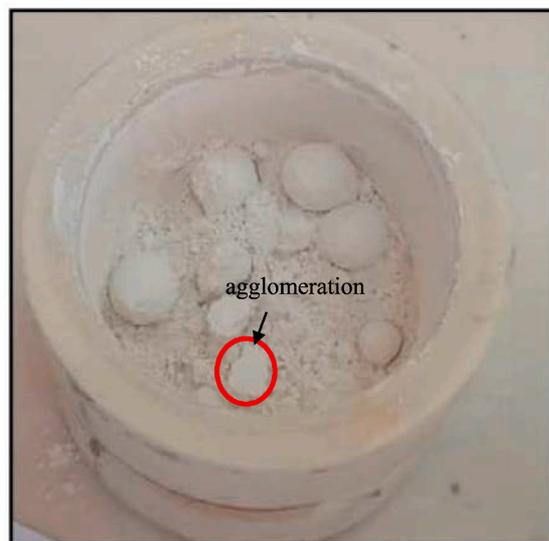
Fig. 3. Eggshell powder after 7 h milling time.
