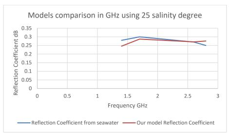
Figure 4. Comparison between low-cost measurement salinity model and our model.
