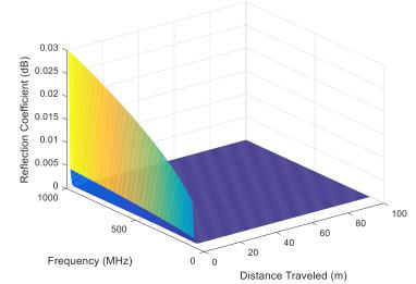
Figure 1. Reflection coefficient at 30 ppt salinity level from 100 MHz to 1 GHz
