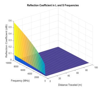
Figure 3 . Reflection coefficient at 25 ppt salinity level from 1 to 10 GHz
