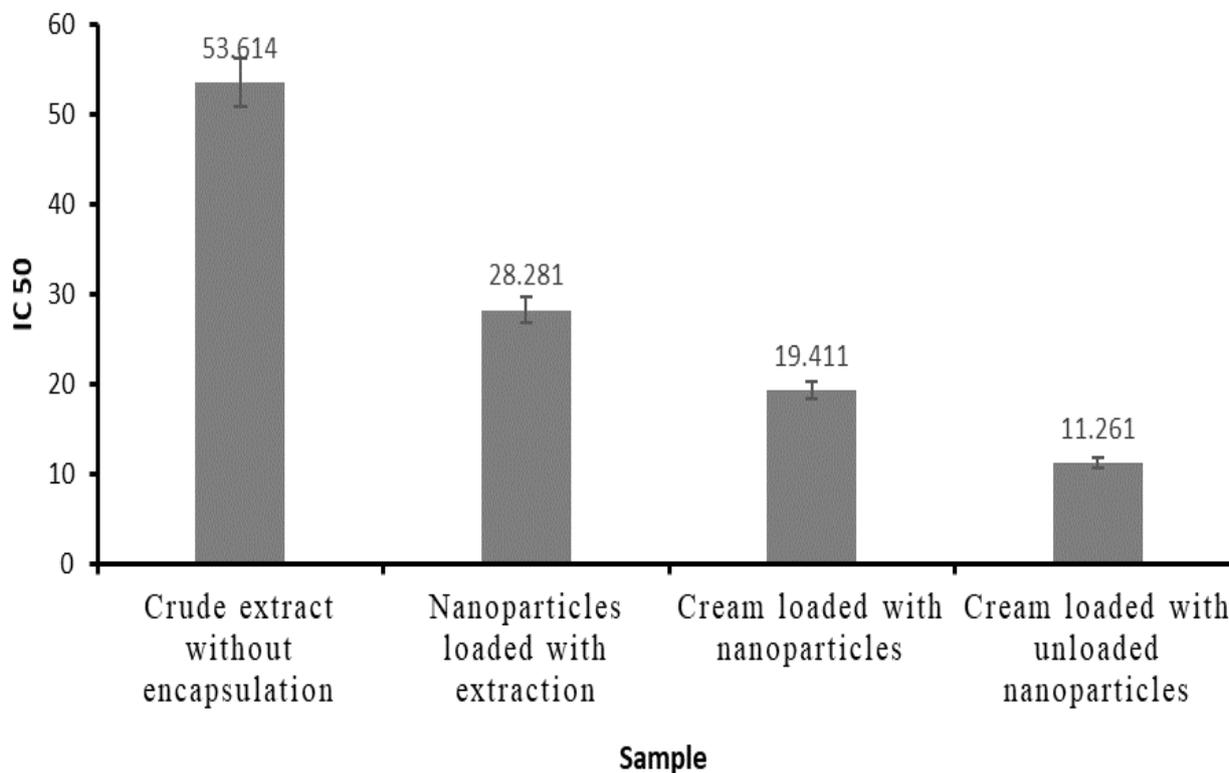
**Figure 5:** Comparison of antioxidant study on the crude extract of *Cymbopogon sp.*, nanoparticles loaded with the extraction of *Cymbopogon sp.*, cream loaded with nanoparticles and cream loaded with unloaded nanoparticles.
