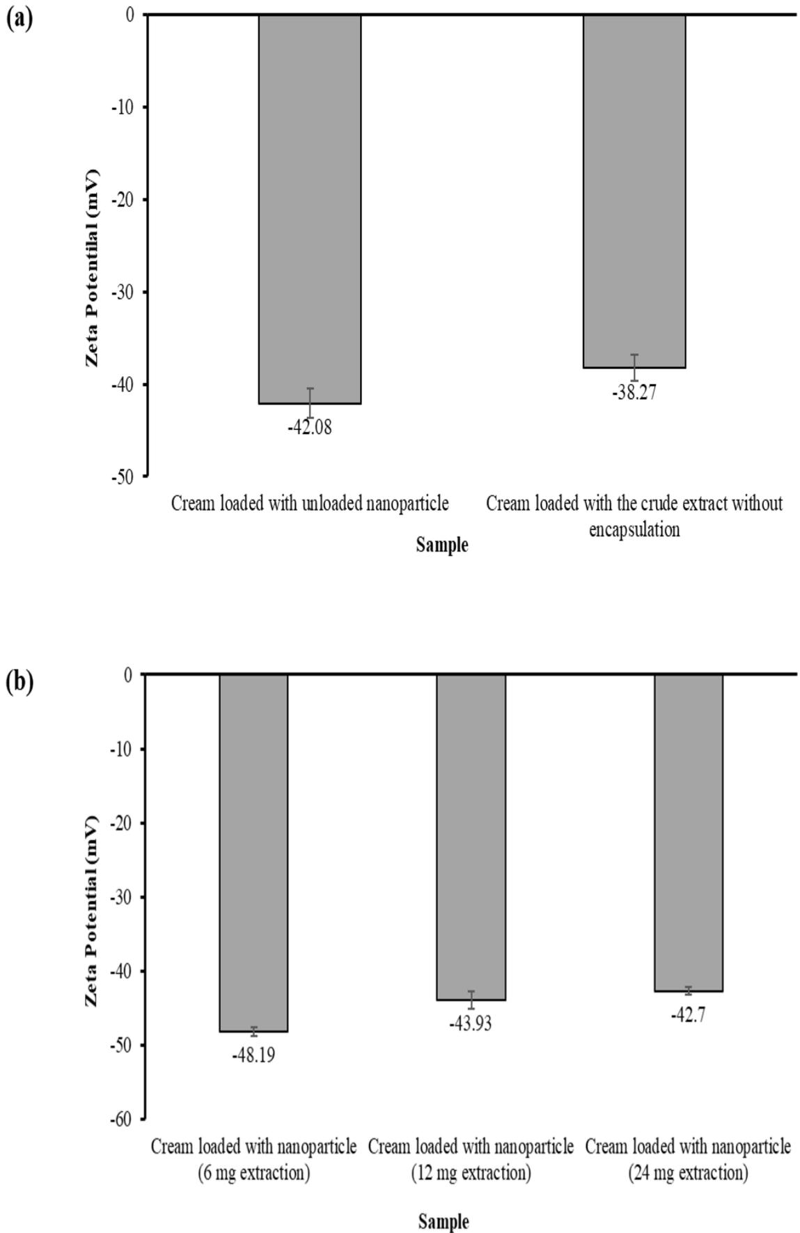
**Figure 3:** Zeta potential of cream loaded with **(a)** unloaded nanoparticles and crude extracts without encapsulation (Mean  $\pm$  SD, n=5); **(b)** nanoparticles of different concentrations of *Cymbopogon sp.* extracts (Mean  $\pm$  SD, n=5).
