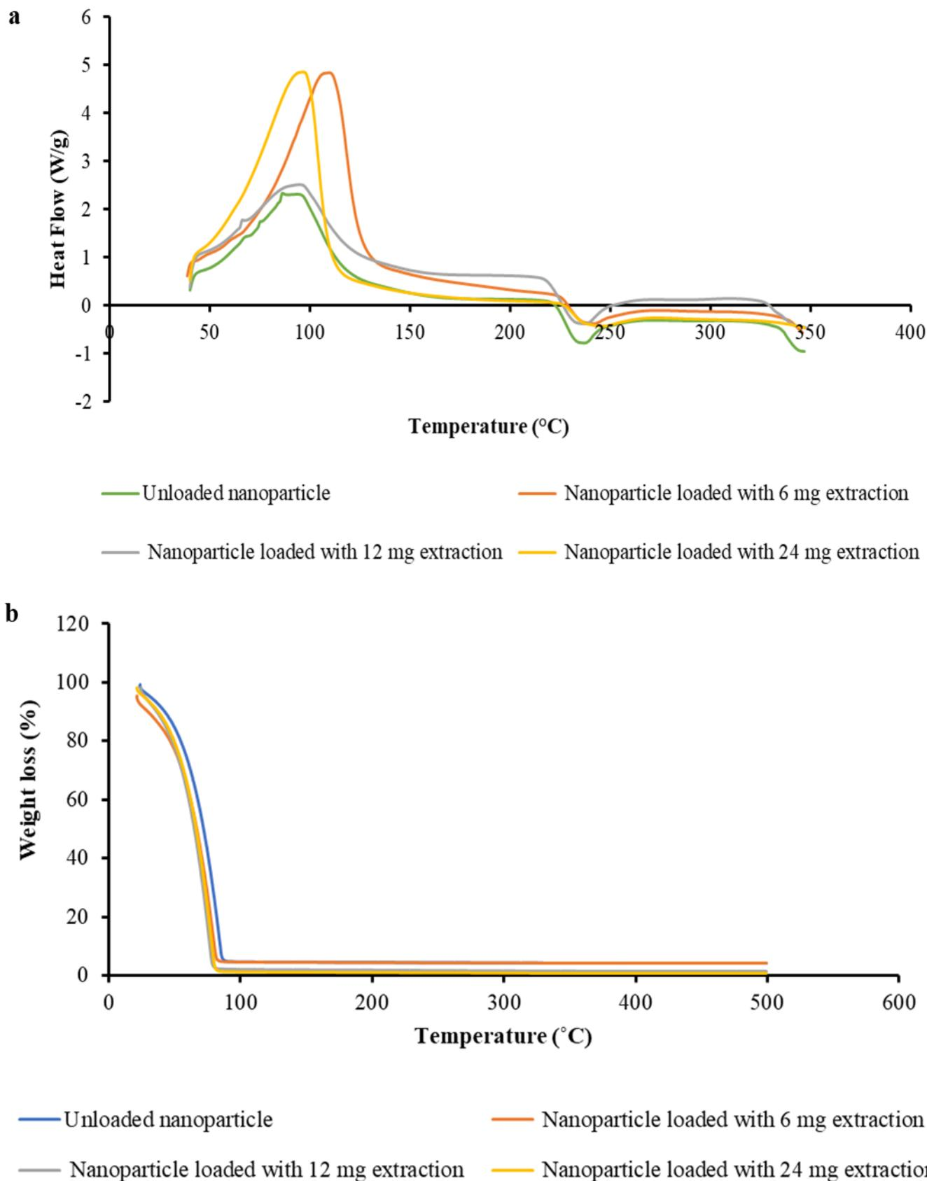
**Figure 1:** Thermal analysis on the prepared nanoparticles samples of different concentrations and controlled samples. **a** DSC thermograms of unloaded nanoparticles and nanoparticles of different concentrations of *Cymbopogon sp.* extracts; **b** TGA Analysis on unloaded nanoparticles and nanoparticles loaded with different concentrations of *Cymbopogon sp.* extracts.
