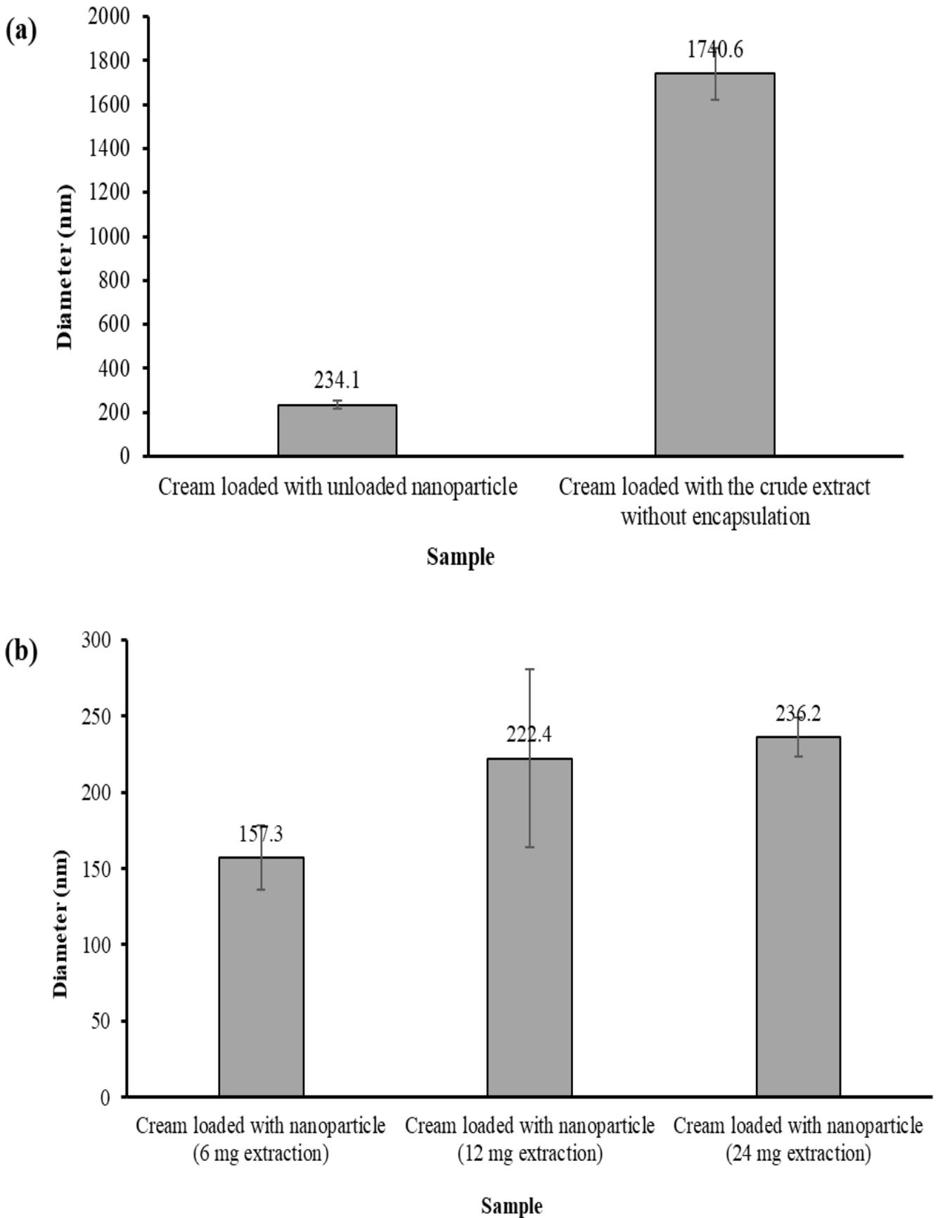
**Figure 2:** The particle size of cream loaded with (a) unloaded nanoparticles and crude extracts without encapsulation (Mean  $\pm$  SD, n=5); (b) nanoparticles of different concentrations of *Cymbopogon sp.* extracts (Mean  $\pm$  SD, n=5).
