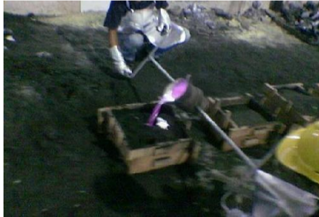
Figure 3.5 g Pouring melt aluminum
