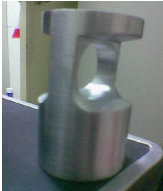
Figure 4.0 b Machined piston
