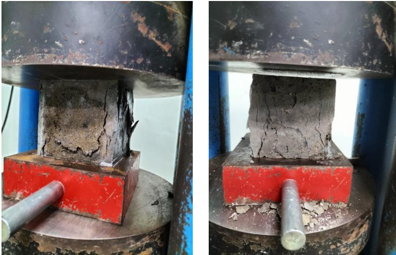
Figure 4.3: Compressive Strength Test Failure
