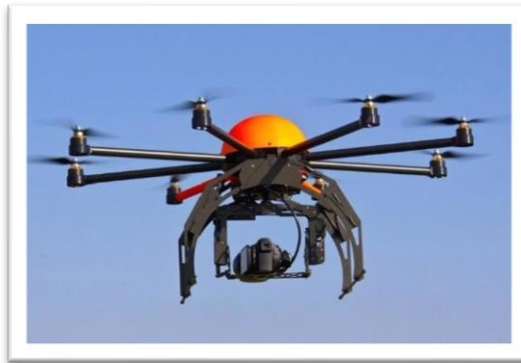
Figure 2.2 Drone and photogrammetric surveying combine photos of the same spot on the ground taken from various angles to produce detailed 2D and 3D maps
