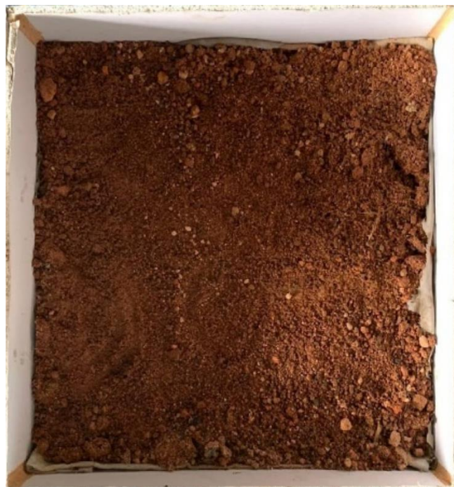
Figure 3.7 The burnt soil substrate layer in green roof system
