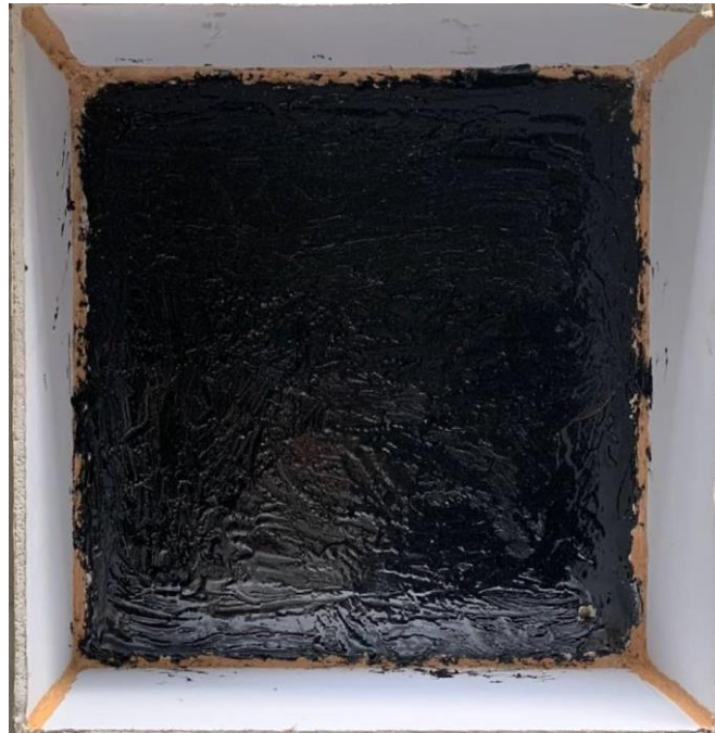
Figure 3.10 The bitumen waterproofing layer at the bottom layer
