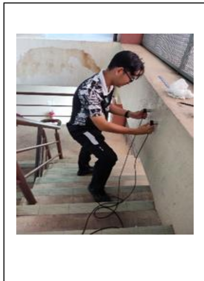
Figure 3.5 Testing UPV on beams at the FKASA building
