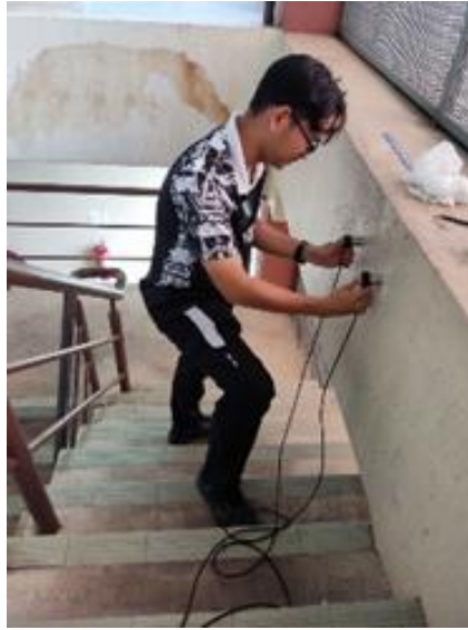
Appendix D: Picture of testing UPV on Beam 1
