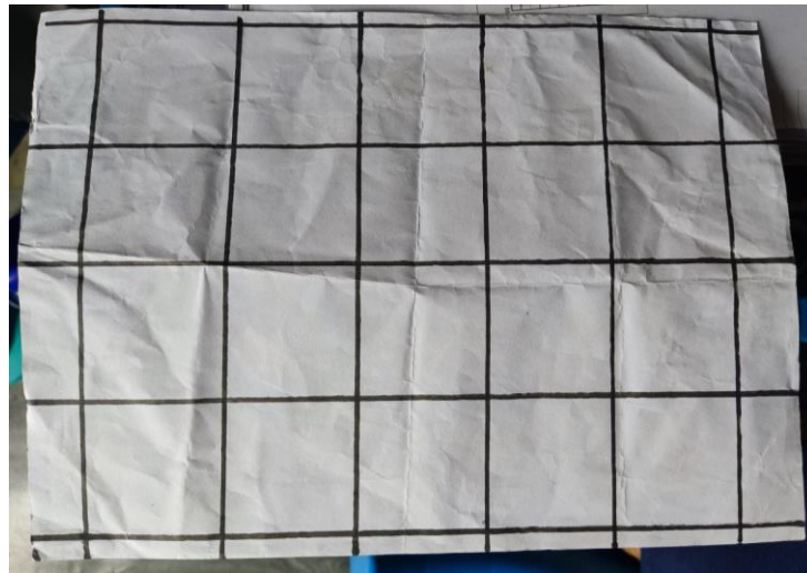
Figure 3.4 Grid for rebound hammer test
