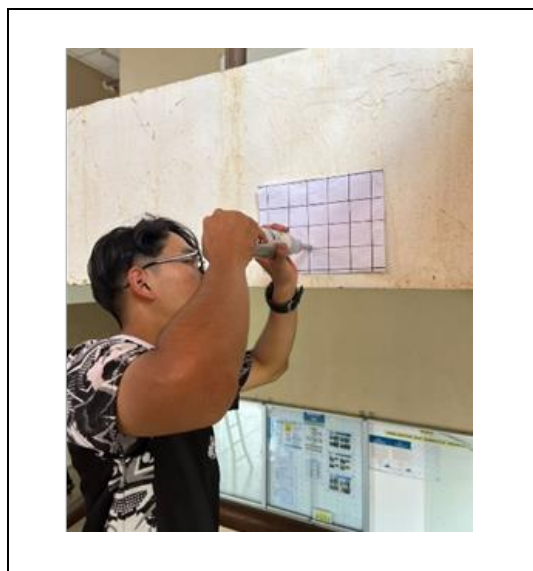
Figure 3.6 Tested rebound hammer on beams at FKASA building
