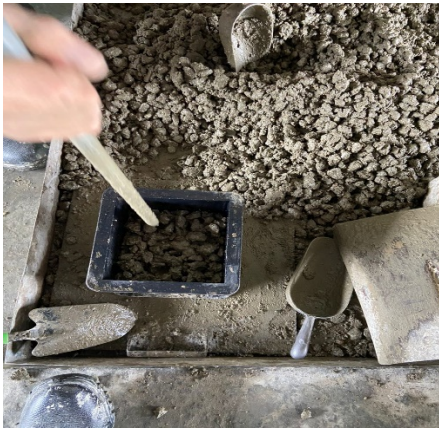
Tapping 25 times on the mould Compacting the concrete mix design
