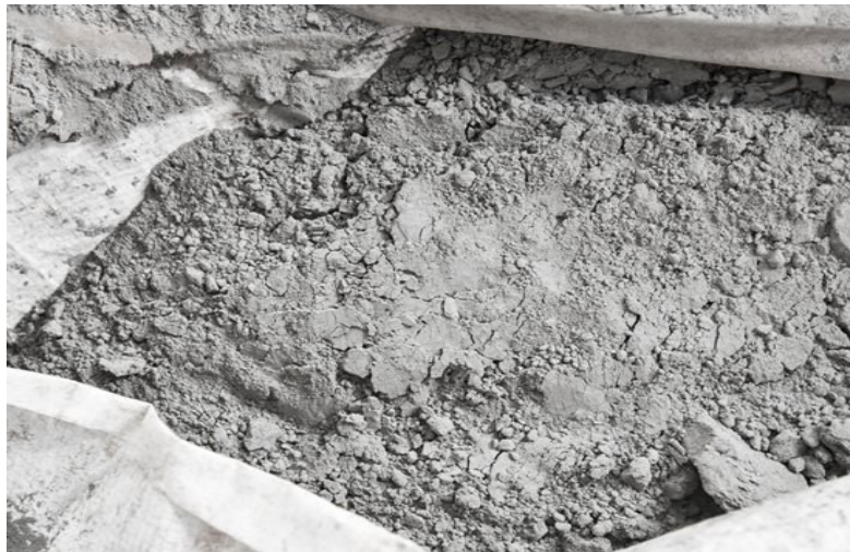
Figure 3.2 Ordinary Portland Cement
