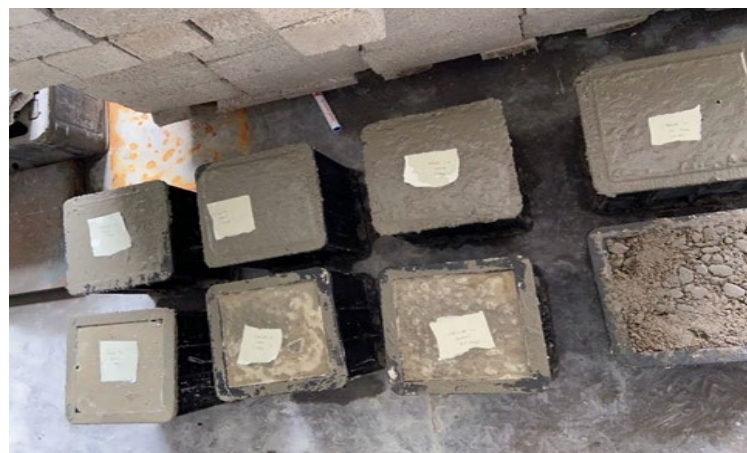
Figure 3.6 The concrete cube in the mold after casting
