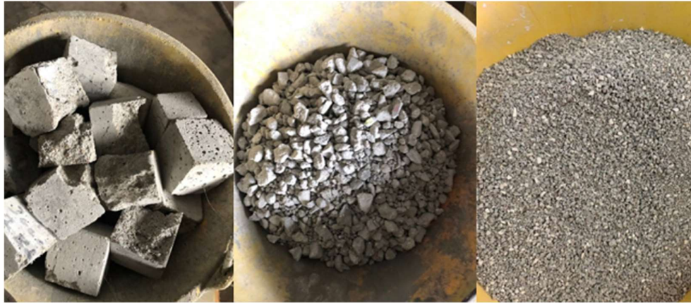
Figure 3.3.1 ii : The crushing process of concrete waste from cube to fine aggregate
