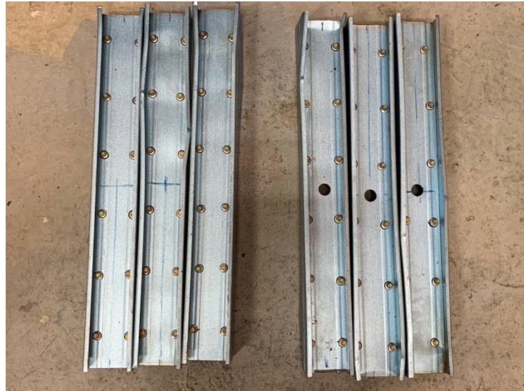
Figure 4.7 Final result of buckling shape behaviour
