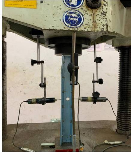
Figure 3.5 The placing of transducer from front view
