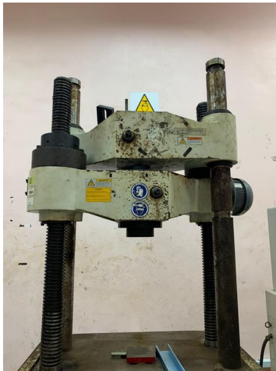
Figure 3.4 Shows the UTM machine , a machine we used to do the axial load test
