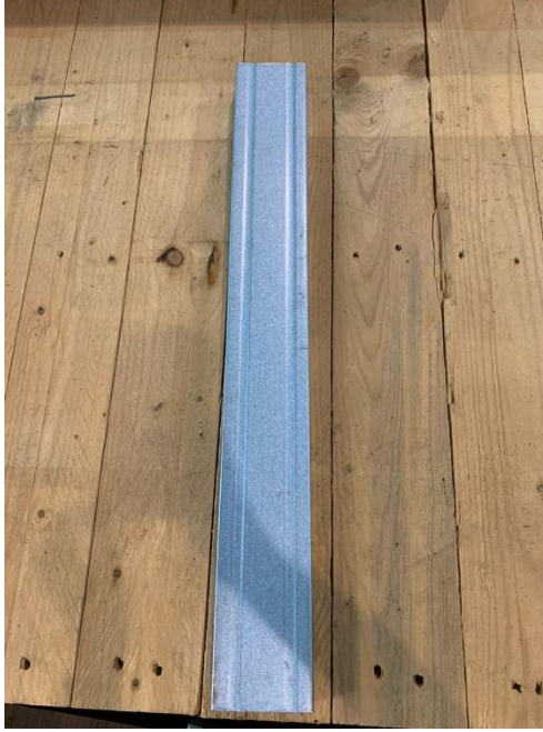
SINGLE C-SECTION WITHOUT AN OPENING OVERVIEW
