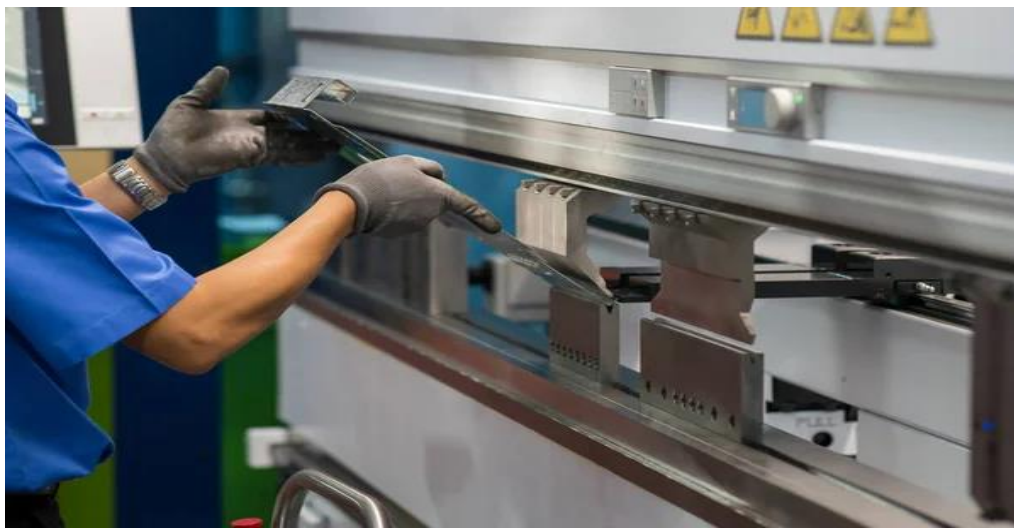
Figure 2.4 Press braking method. Sources : MechStuff
