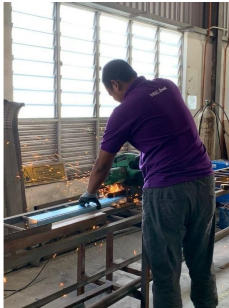
Figure 3.2 Shows the PIC cut half of the specimen to 600mm
