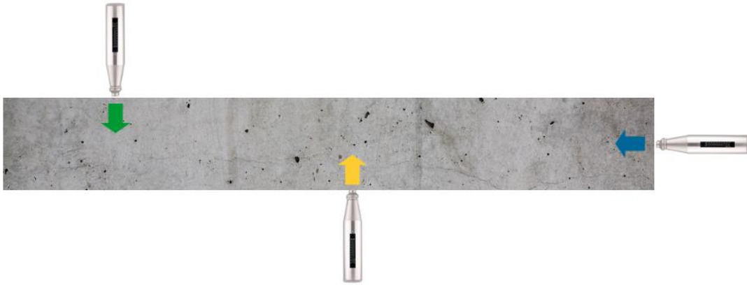
Figure 2.2 Rebound hammer direction
