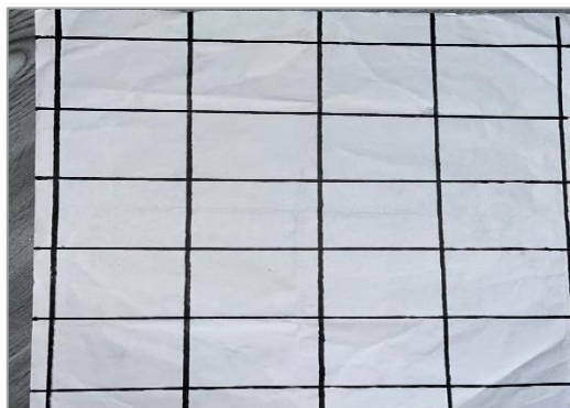
Figure 3.10 Grid size 500 mm x 500 mm on sheet paper for rebound hammer testing
