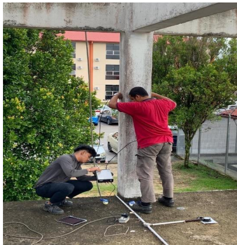
Figure 3.8 Direct method on mid-height of the column
