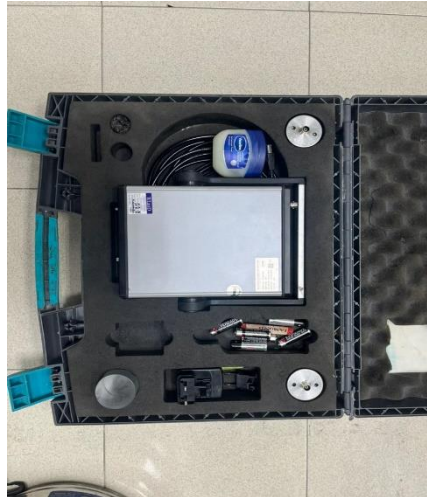
Figure 2.3 Proceq's PUNDIT Source: Pundit Lab. Ultrasonic Pulse Velocity Tester (2020)
