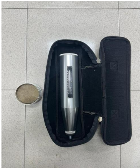
Figure 3.9 Rebound hammer and grindstone
