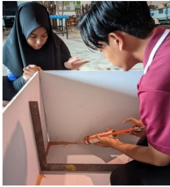
Figure 3.7 Process of placing the sealant
