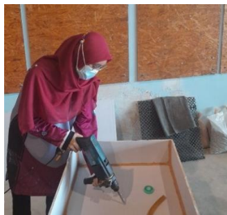
Figure 3.9 Process of drilling a hole to insert pipe
