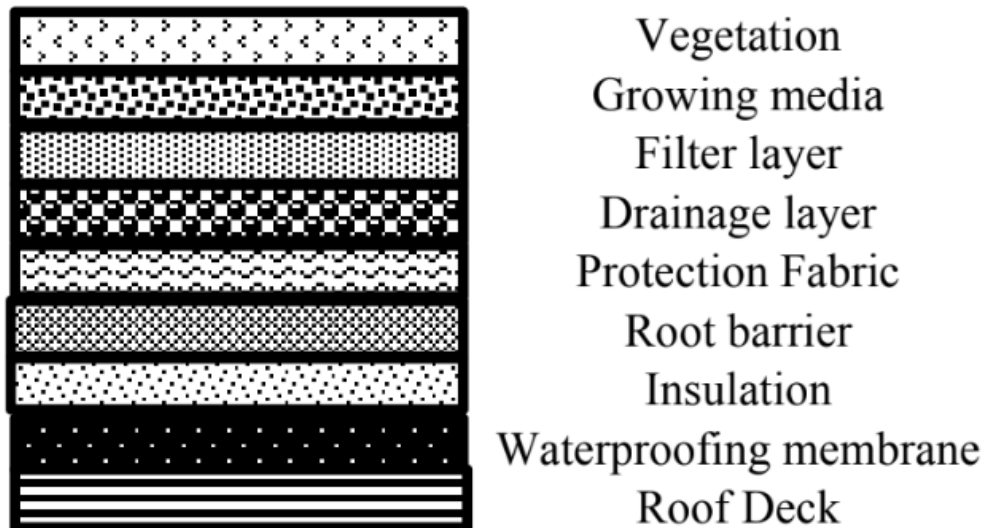
Figure 2.6 Structure of green roof system
