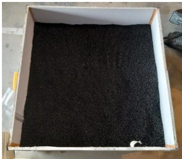
Figure 3.20 Drainage layer of recycled waste green roof
