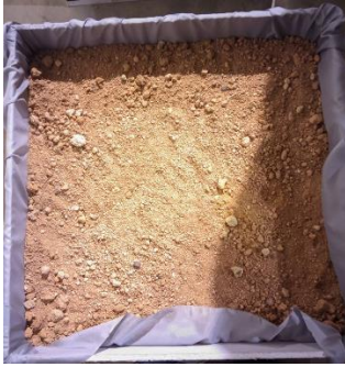
Figure 3.17 Substrate layer of green roof model
