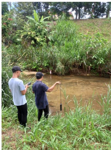
Collection of data using Handheld Multiparameter
