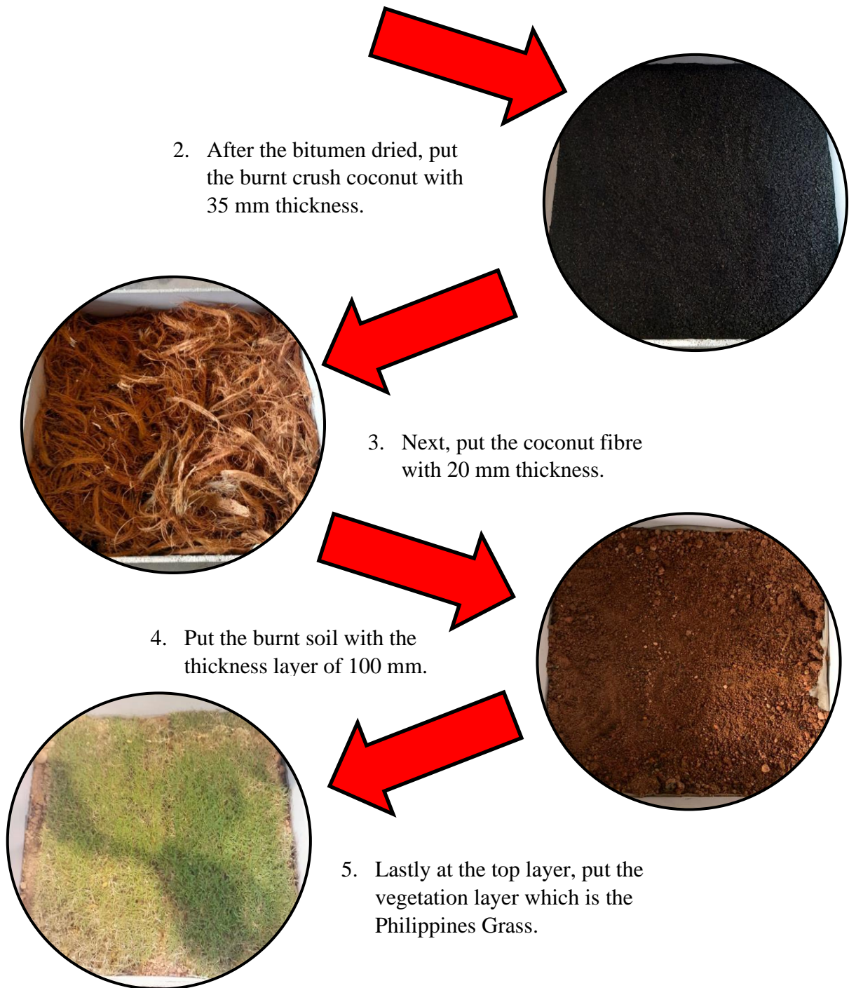
Figure 3.13 Construction of Green Roof Recycled Waste (Layer)
