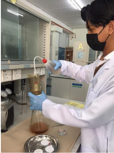
The FYP student was washing the funnel with distilled water in TSS test
