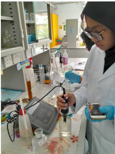
The FYP student was taking the reading of BOD in BOD test
