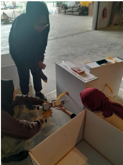
The FYP student was sealing the suction pipe into the roof model
