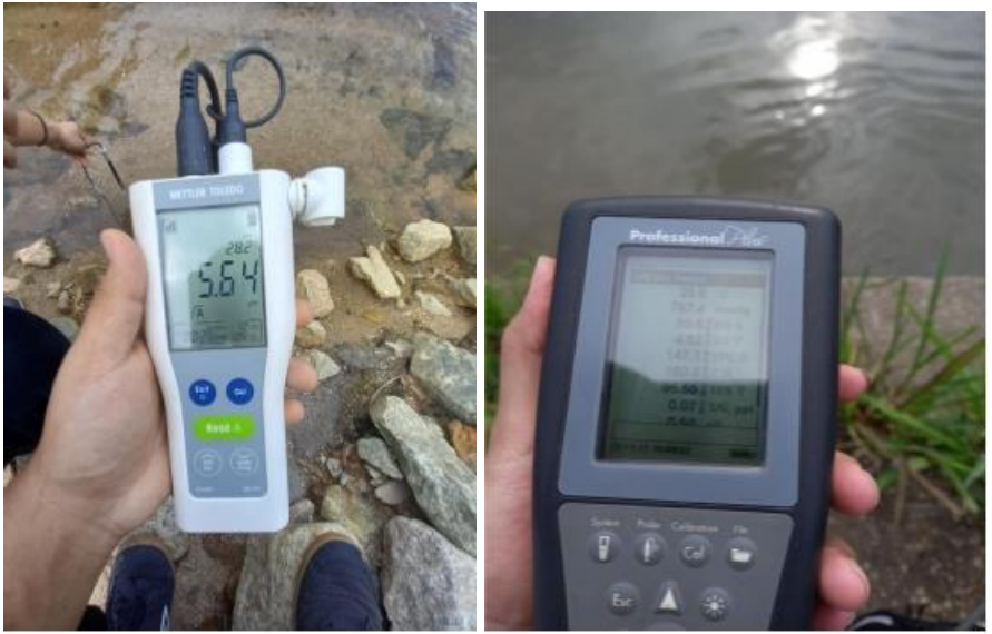
Picture 6: Shows the uses of a PH meter and a Handheld water multi-parameter.
