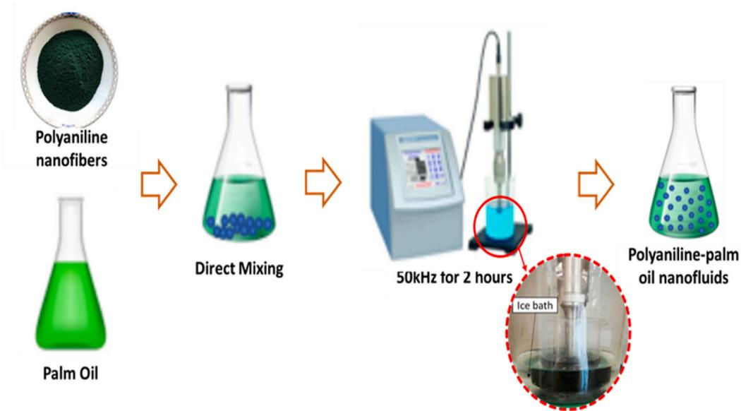
Fig. 3. Illustration of polyaniline-palm oil nanofluids formulation method.
