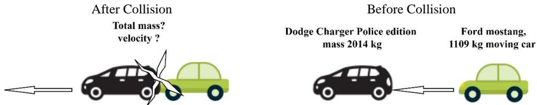
Figure 8. Schematic of collision simulation
