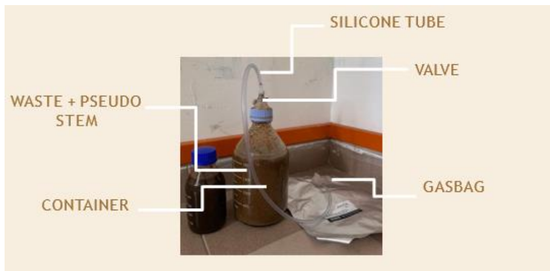
Figure 3.2 The set-up of production of methane from fruit and pseudo stem banana wastes
