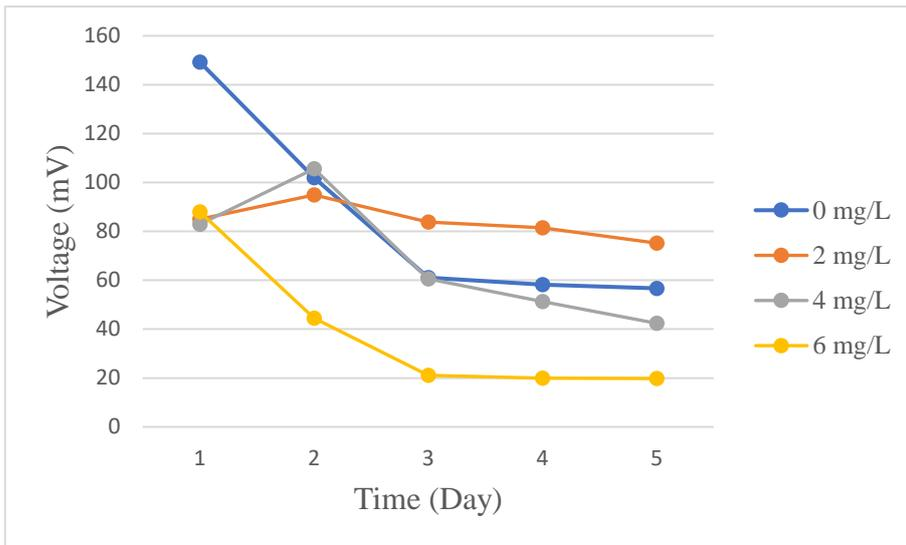
Figure 4.1 Voltage variation over time for different dosage of WPOS throughout the MFCs test.
