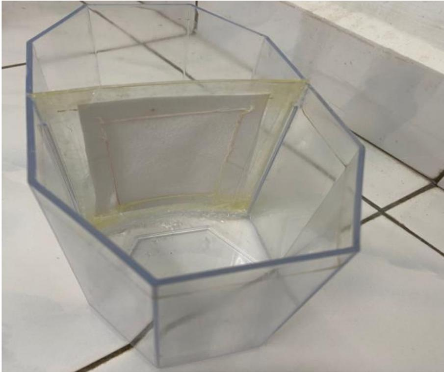
Figure 3.5 Modification of filter paper as separator
