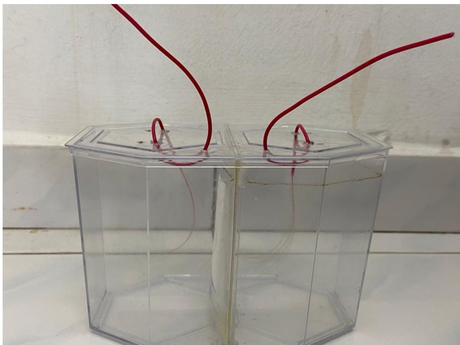
Figure 3.4 Dual chamber of MFC by using copper as electrode
