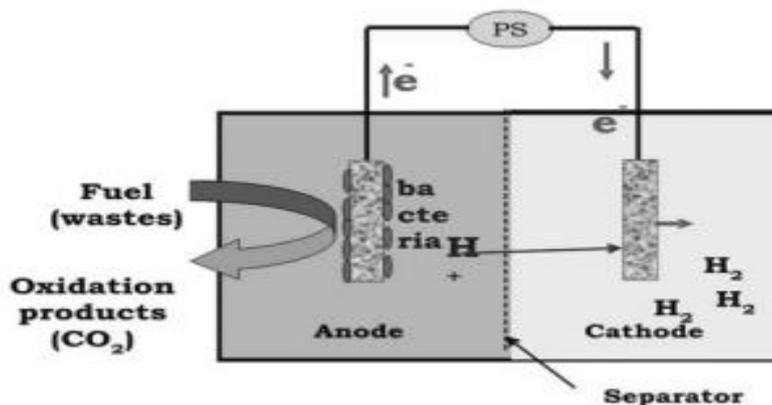
Figure 2.4 Basic principle of Microbial Fuel Cell
