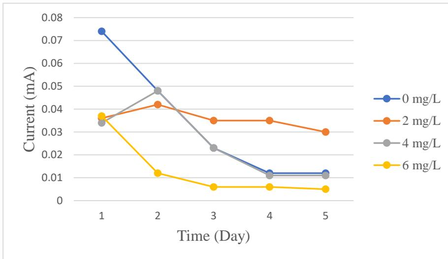
Figure 4.2 Current variation over time for different dosage of WPOS throughout the MFCs test.
