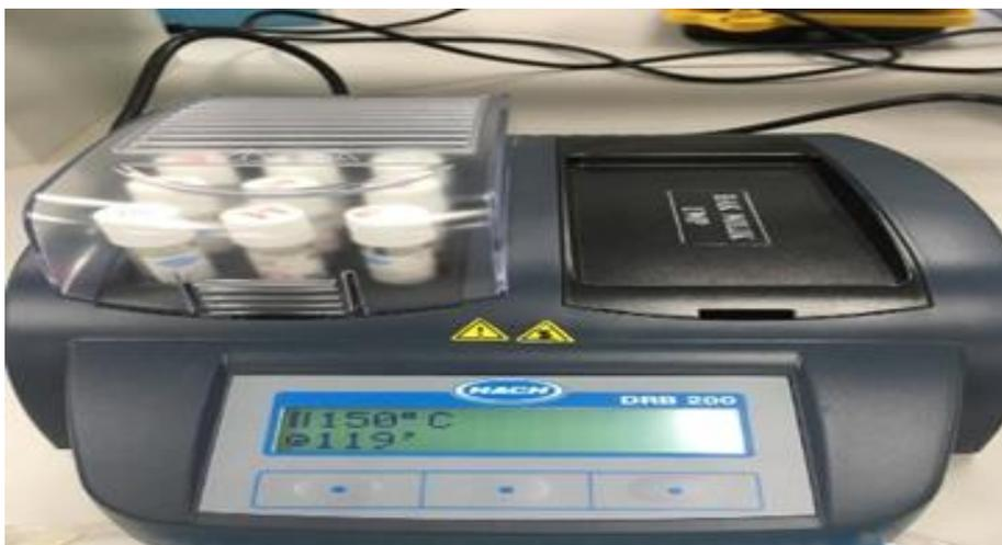
Figure 3.8 Several mixtures of samples with COD digestion reagent
