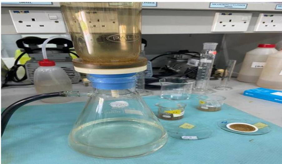
Figure 3.8 Apparatus used in TSS test
