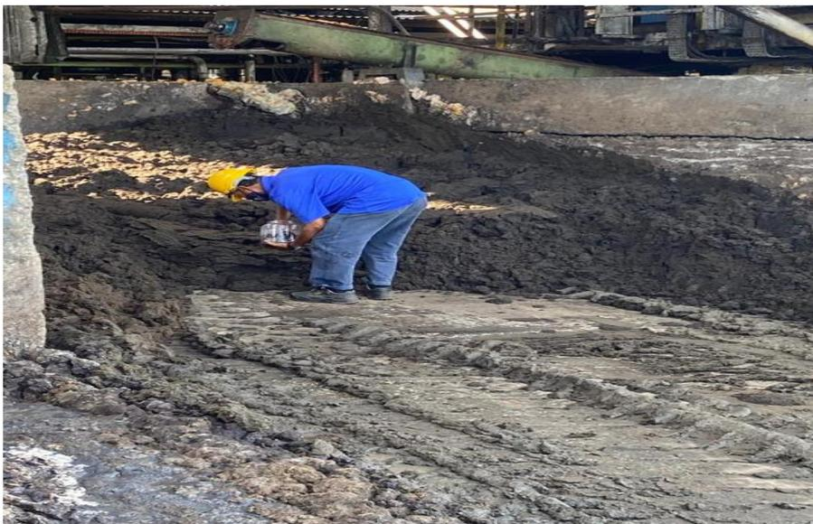
Figure 3.3 Sample of wet palm oil sludge from Kilang Sawit
