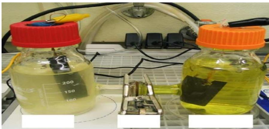
Figure 2.5 Simple Double Chamber Microbial Fuel Cell
