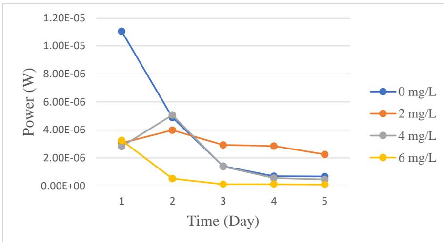
Figure 4.3 Power variation over time for different dosage of WPOS throughout the MFCs test.
