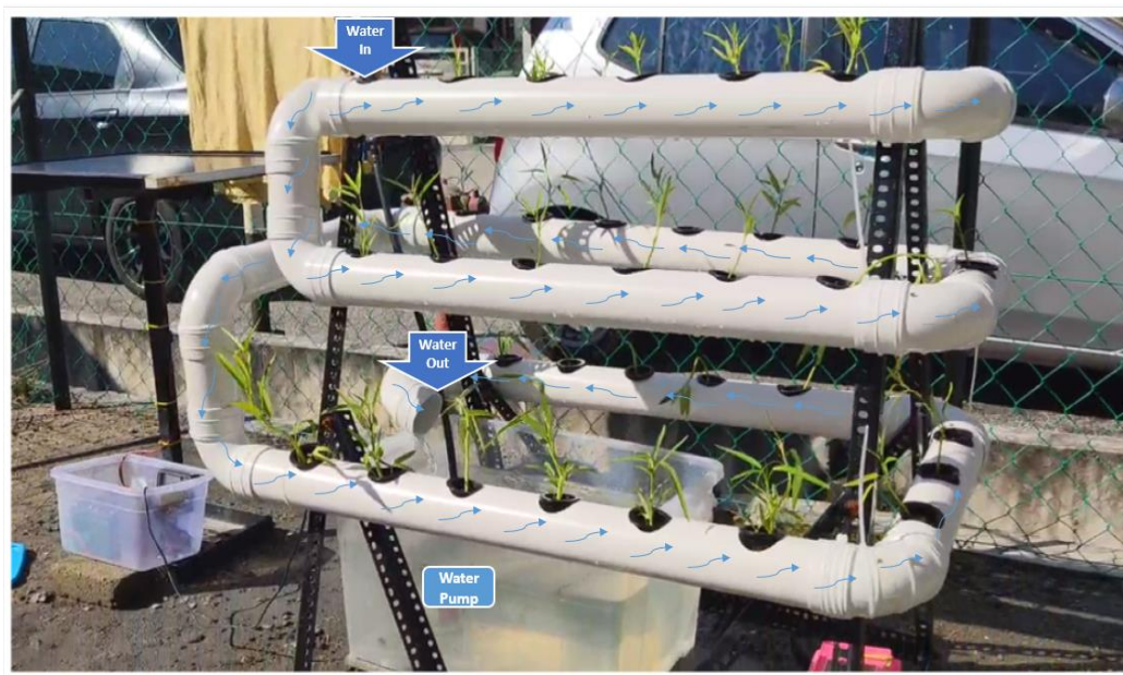
Figure 3.2 Complete System of In-house Solar Powered Automatic Irrigation System with Aquaponics' Concept
