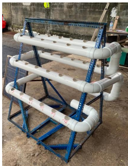
Figure 3.11 Completed Piping Section on Main Structure
