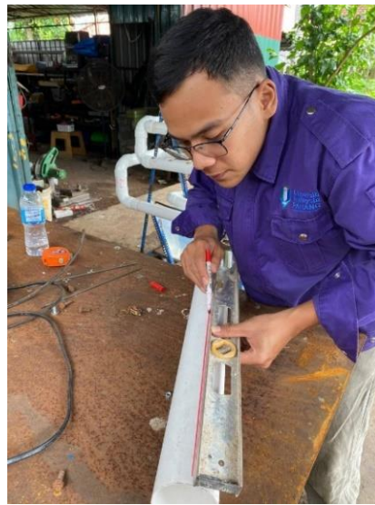
Figure 3.10 Measuring Process Before Drilling The Holes
