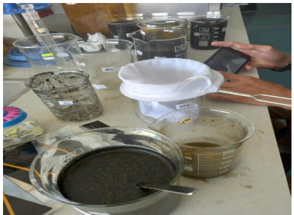
Figure B8: Filtered of Wastewater sample
