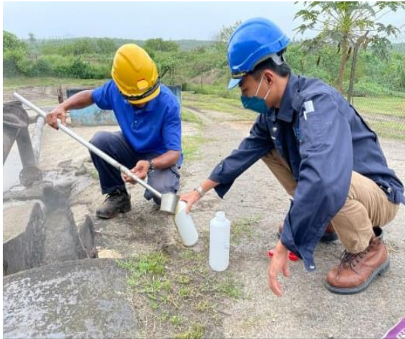
Figure B5: Collected of Wastewater Sample
