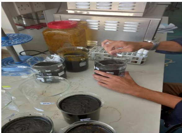
Figure B7: wastewater sample mixed with Activated Carbon
