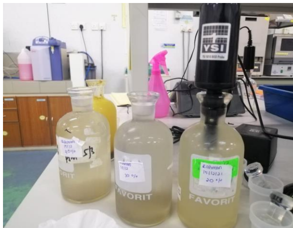
Figure B10: BOD test
