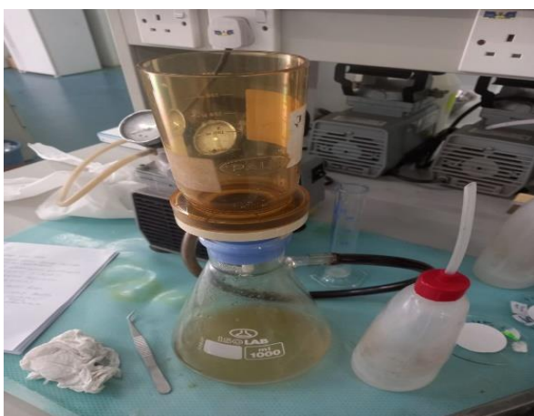
Figure B9: Total Suspended Solids test
