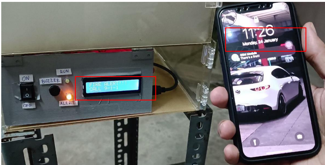
Figure 21: Displayed Information on LCD and SMS During ALERT State (Fire Occurs)
