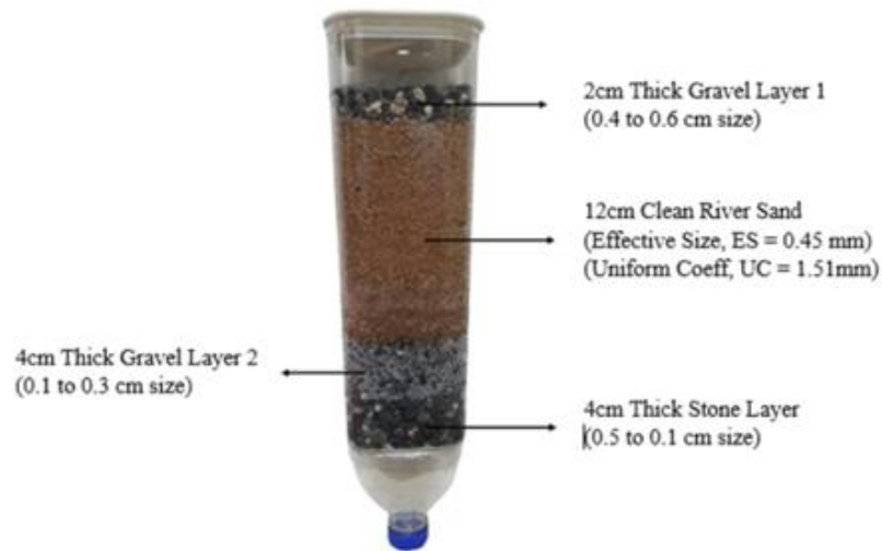
Figure 4.7: Fabricated Lab-scale Sand Filter
