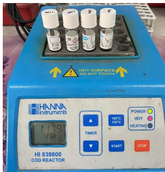
Figure 3.2 HI 839800 COD reactor
