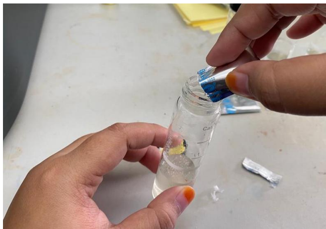
Figure 3.4 Adding Ammonia Salicylate Powder into the sample cell
