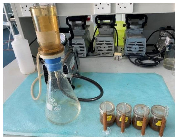
Figure 3.3 Apparatus set up for TSS
