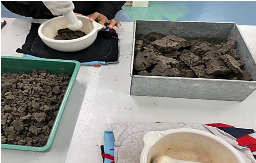
Appendix I: Crushing and sieving of carbonized palm oil mill sludge (POMS).
