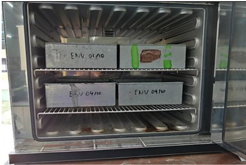
Appendix C: Drying process of palm oil mill sludge (POMS) in oven.
