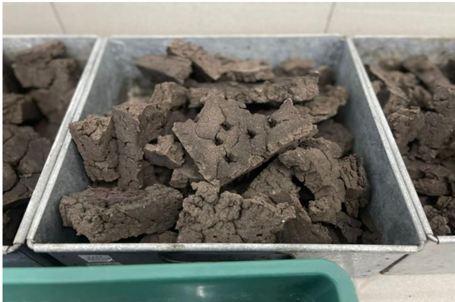
Appendix D: Dried palm oil mill sludge (POMS).
