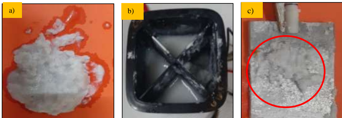
Figure 4.10: The white gelatinous precipitate, Aluminium Hydroxide Al(OH)_3 (a) the removed Aluminium Hydroxide Al(OH)_3 , (b) the formation of Aluminium Hydroxide Al(OH)_3 after run for 48 hours and (c) the formation of Aluminium Hydroxide Al(OH)_3 that sticking.
