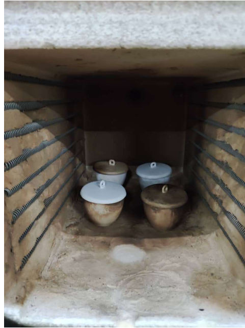
Figure 5: Sieved WH in furnace for pyrolysis process
