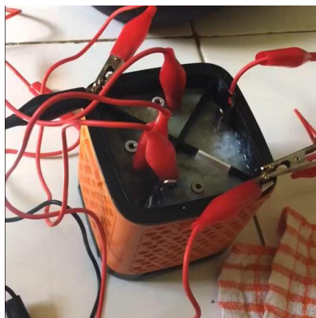
Figure 4.1 Al(OH)_3 and Hydrogen Gas Formation in Al – air Fuel Cell
