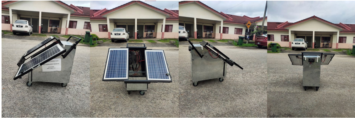
Figure 3.12 Solar panels faced four different orientations which are East, North, West and South according to the sequence.
