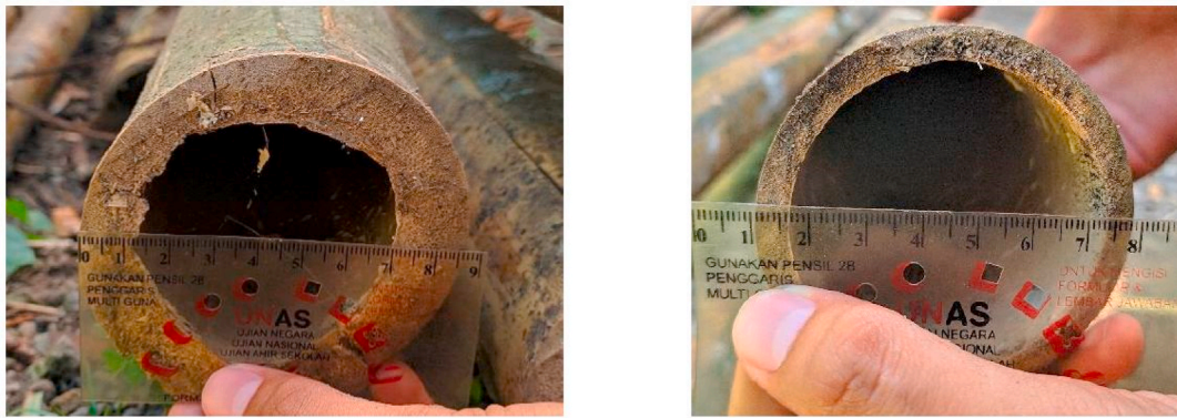
(a) Diameter=0.07 m, Radius=0.035 m, Volume = 0.33 m 3 (b) Diameter=0.085 m, Radius=0.0425 m, Volume=0.4 m 3
