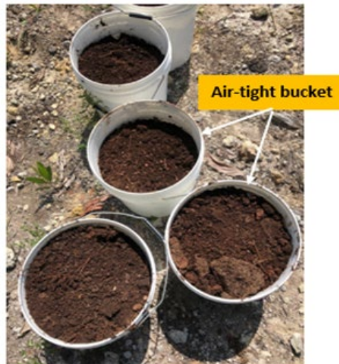
Fig. 2. The peat soil samples collection (air-tight bucket)
