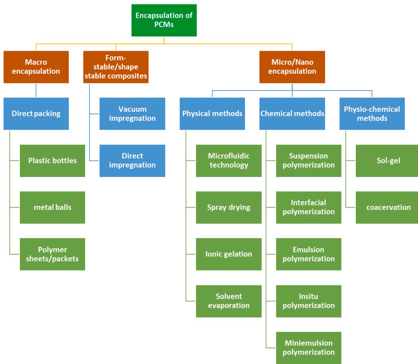
Fig. 3. The classification of encapsulation methods for phase change materials.
