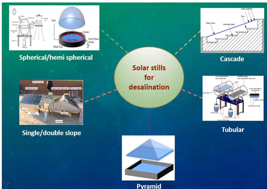
Fig. 12. Pictograph Illustrating Different Types of Solar Stills for Water Treatment (Desalination).
