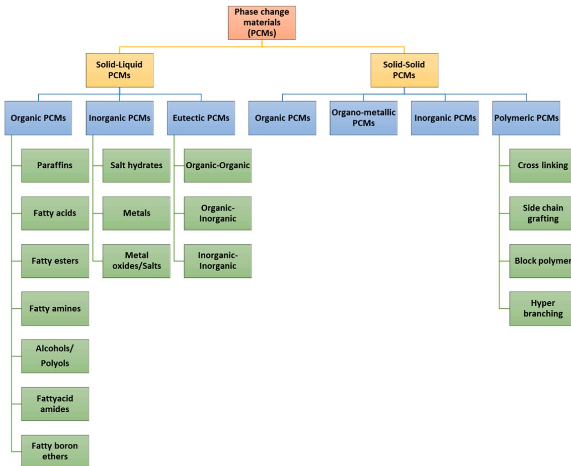
Fig. 2. The broad classification(up-to-date) of the phase change materials based on their phase change behavior and composition.
