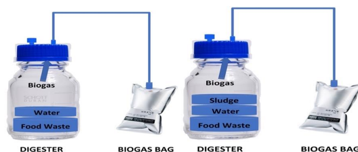
Figure 1 Set up of anaerobic digestion of food waste with and without sludge
