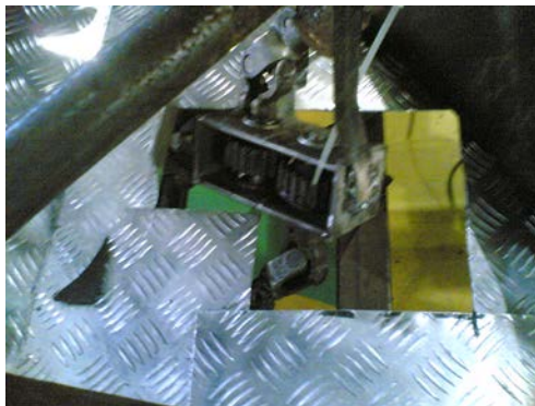
Figure 3.9:- Gearbox placement at the buggy
